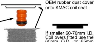
If smaller 60-70mm I.D. Coil overs fitted use the 60mm O.D. or 65mm O.D. elastomer KMAC seats supplied.
