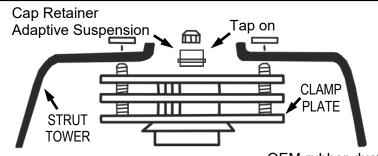
KMAC BUMP STOP if lowering can cut top section of bump stop off to increase shock travel/absorption.
