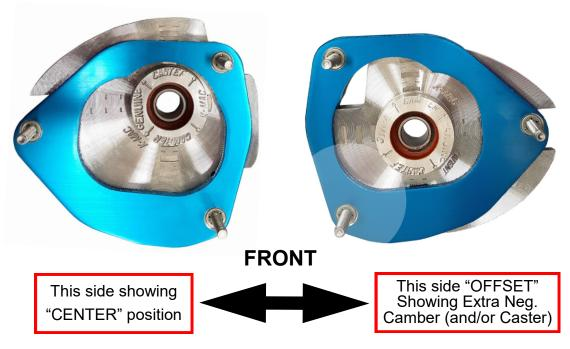
(IF INNER TIRE WEAR) SWAP SIDES — CENTER HOLE OFFSET OUTWARDS. And to REAR for Pos. Caster.
