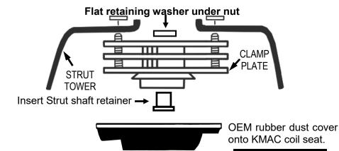
KMAC BUMP STOP if lowering can cut top section of bump stop off to increase shock travel/absorption.
