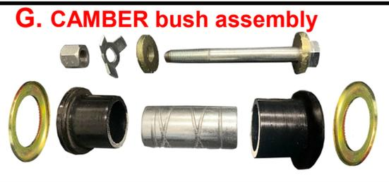
**H.** For ease of bolt entry preferably rotate bush 'D' holes to 12 o'clock position. (Flat then is to Top).
