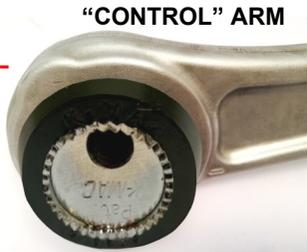
C. Lower control arm sufficient to expose Bush.
