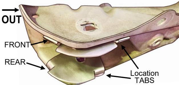
CHECK (Front or Rear) So Tabs fully seated. See back of sheet cover
