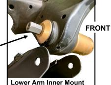
E. Insert the new K-MAC elastomer bushes. Now lubricate the steel inner bushes (only) with silicone grease supplied and insert.
