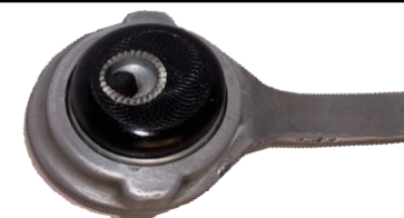
New Adj. Bush installed with insulator caps as in step F
