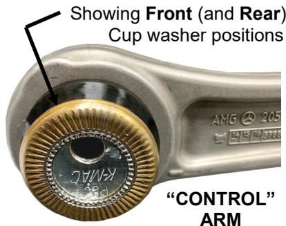
**F** Clean hole and insert the 2 elastomer bushes for each arm. Then use grease supplied to lubricate the KMAC steel bushes (only) and insert with hole at 12 O'clock.
