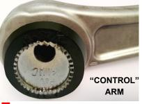
P. Clean hole and insert the 2 elastomer bushes for each arm. Then use grease supplied to lubricate the KMAC steel bushes (only) and insert with hole at 12 O'clock
